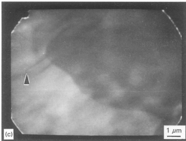
Figure 3 Growth of the normal mode observed during transformation from austenite to ferrite in an Fe-0.71 wt % C alloy. The spikes indicated by the arrow head as a common point of reference, are likely to be stacking faults in the austenite. (a) Schematic diagram of the interface positions in b-d. (b) The ferrite growing from the top-right position. (c) The same interface recorded 1 s after (b). (d) Again as (b) but now after 3 s. The scale marker indicates a length of 1 \mu\text{m} .
